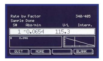
See the curve, then calculate kinetic results based on the entire read time or
