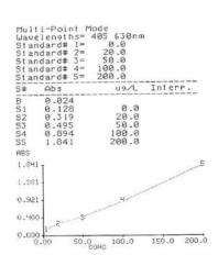
For each run, choose a new curve or use a stored curve with options to modify multi-point curves and revert to previous curve.
